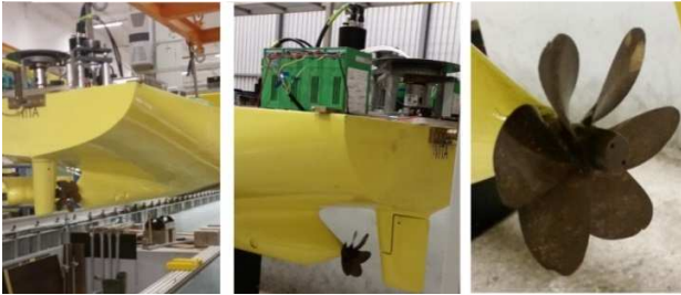
FIGURE 3: SINGLE PROPELLER AND SINGLE SEMI-BALANCED RUDDER INSTALLED ON THE SHIP MODEL
