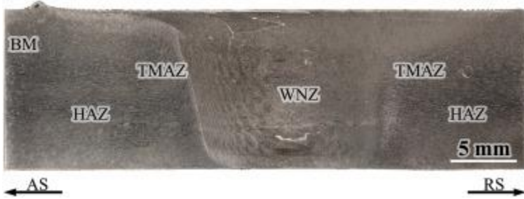
Fig. 3. Photograph showing the four macroscopic weld zones.
