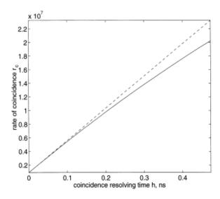
Fig. 3. The rate of coincidence registration as a function of the coincidence resolving time *h*. Solid and dashed lines represent the exact and approximate results, respectively. The following set of parameters are used:  $\eta_s = \eta_i = 0.1$ ,  $\beta = 0.5$ ,  $\lambda = 1.8 \times 10^8$  photons/s and  $\mu_s = \mu_i = 2 \times 10^9$  photon/s.
