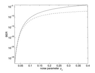
Fig. 8. The bit-error rate (BER) as a function of the coincidence-noise parameter  $\rho_c$ . Solid and dashed lines represent the exact and approximate results, respectively. The following set of parameters are used:  $\eta_s = \eta_i = 0.1$ ,  $\beta = 0.5$ , h = 1 ns, and  $\lambda = 1.8 \times 10^8$  photons/s. The coincidence parameter is varied by changing the background noise flux  $\mu_i$ .
