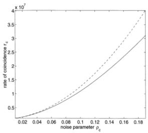
Fig. 1. The rate of coincidence registration as a function of the accidental noise parameter  $\rho_c$ . Solid and dashed lines represent the exact and approximate results, respectively. The following set of parameters are used:  $\eta_s = \eta_i = 0.1$ ,  $\beta = 0.5$ , h = 1 ns, and  $\lambda = 1.8 \times 10^8$  photons/s. The noise flux is varied so that the parameter  $\rho_c$  ranges from 0 to 0.2.
