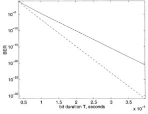
Fig. 9. The bit-error rate (BER) as a function of the bit duration *T*. Solid and dashed lines represent represent exact and approximate results, respectively. The following set of parameters are used:  $\eta_s = \eta_i = 0.1$ ,  $\beta = 0.5$ ,  $\mu_i = 2.0 \times 10^9$  photons/s, and  $\lambda = 1.8 \times 10^8$  photons/s.
