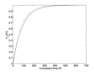
Fig. 5. The probability distribution function, as a function of the normalized time t/h, of the time between successive coincidence events. Solid and dashed lines represent the exact and approximate results, respectively. The following set of parameters are used:  $\eta_s = \eta_i = 0.1$ ,  $\beta = 0.5$ , h = 1 ns, and  $\lambda = 1.8 \times 10^8$  photons/s. The noise parameter  $\rho_c$  is 0.1.
