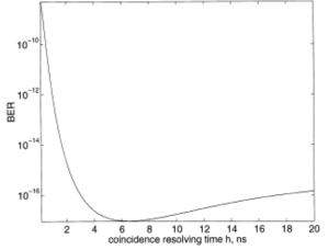
Fig. 11. Exact bit-error rate (BER) as a function of the coincidence resolving time *h*. Other parametrs are the same as those corresponding to Fig. 10.
