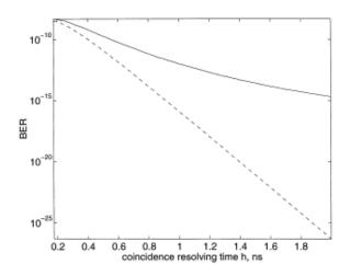
Fig. 10. The bit-error rate (BER) as a function of the coincidence resolving time *h*. Solid and dashed lines represent results obtained using the exact and approximate expressions, respectively, for the rate of coincidence. The following set of parameters are used:  $\eta_s = \eta_i = 0.1$ ,  $\beta = 0.5$ ,  $\mu_i = 2.0 \times 10^9$  photons/s, and  $\lambda = 1.8 \times 10^8$  photons/s. The coincidence-noise parameter  $\rho_c$  is varied by changing coincidence resolving time *h*.
