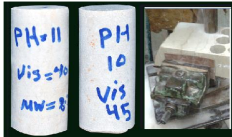
Figure 9. Sample core preparation from Minya marble
