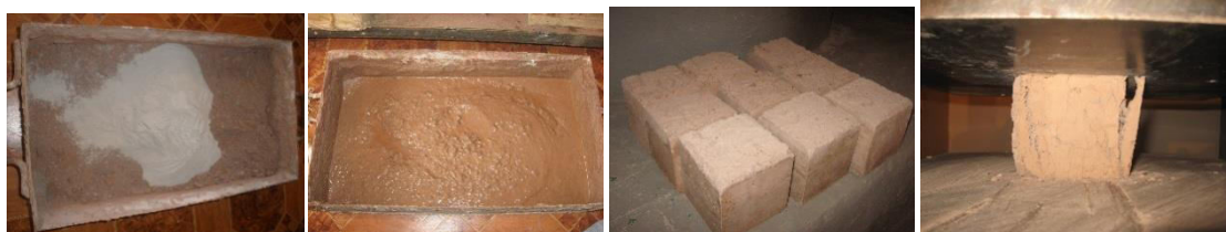
Figure-3. Laboratory studies of preparing the backfill mixtures and testing the samples for strength.
