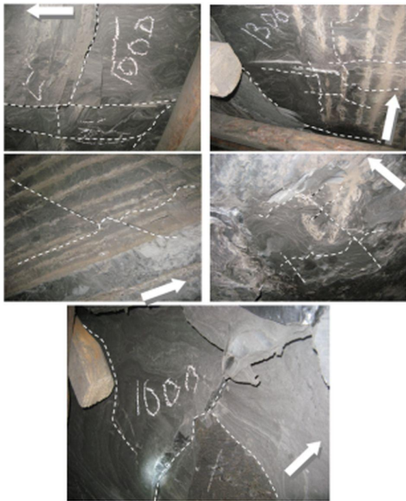
Figure 5. Photos of natural roof outcrops at the distance of 0.8 – 2.0 meters from the seam edge including fracture systems orientation as for the slope length
