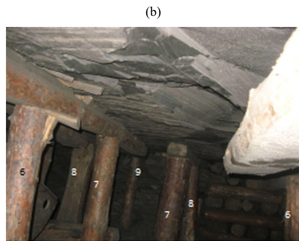
Figure 6. Photos of natural roof outcrops when distance from the seam edge is more than 2 m (photographing direction is from the seam to protective structure; numbers indicate stays across the width of the face area of terminal site)
