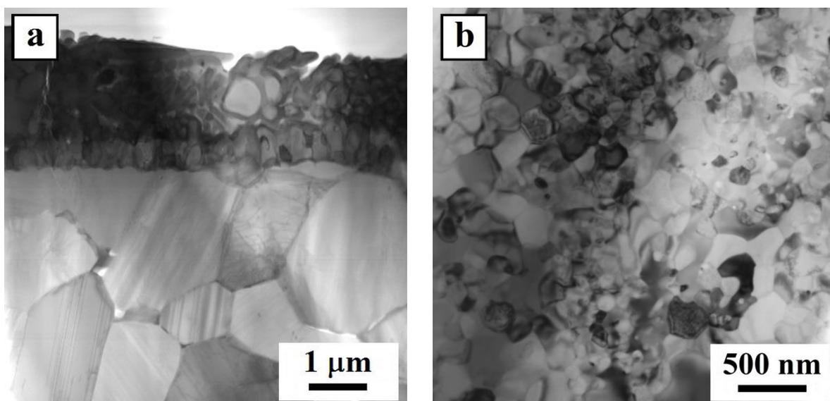
**Figure 5.** The regions of the structure formed during melting and high-speed crystallization, enriched with titanium atoms (regions containing the droplet fraction particle).
