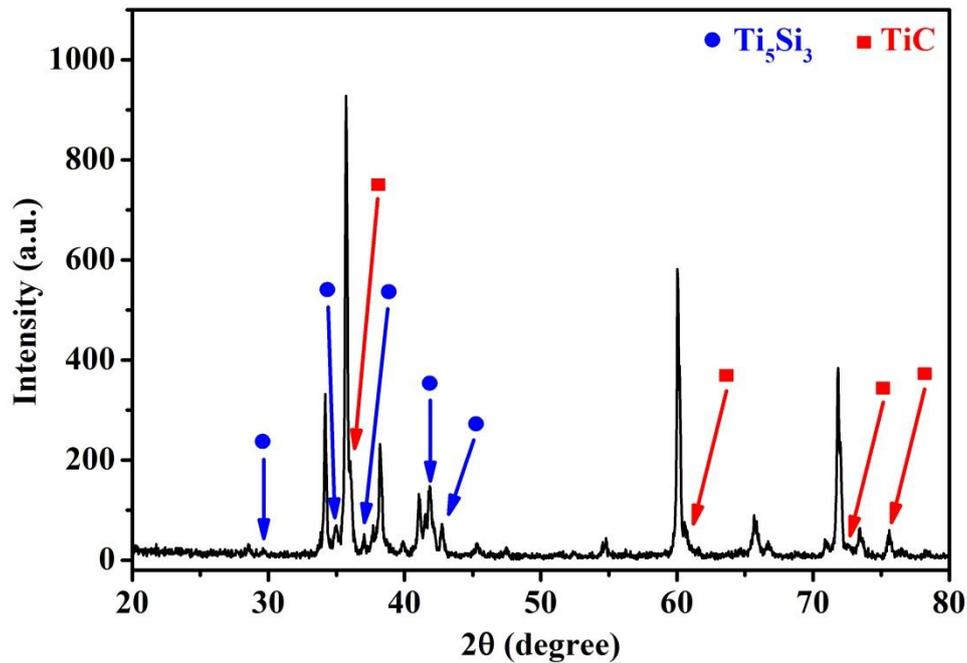
**Figure 4.** XRD pattern obtained from the surface layer of the «film (Ti)/substrate (SiC-ceramics)» system irradiated with an intense pulsed electron beam.
