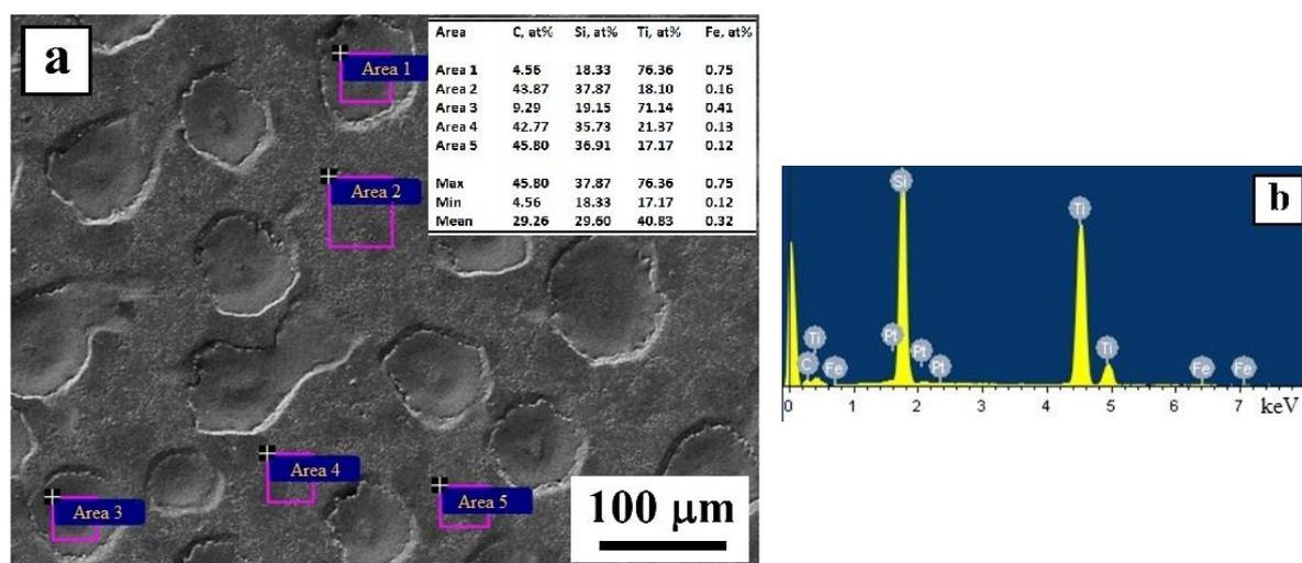
**Figure 3.** Structure of the «film (Ti)/substrate (SiC-ceramics)» system irradiated with an intense pulsed electron beam (a). Areas of analysis of elemental composition are indicated. The table shows the elemental composition of these areas; (b) energy spectra obtained from the sample surface area given in (a).
