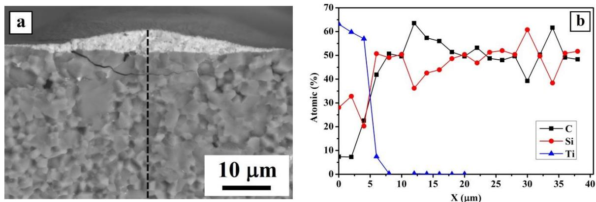
**Figure 6.** Structure of cross-section of the «film (Ti)/substrate (SiC-ceramics)» system (a); (b) the concentration profile of the main elements along the line indicated in (a).
