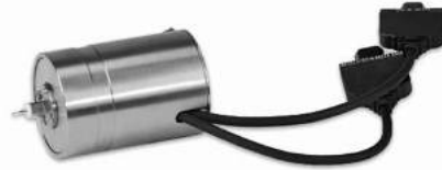
Figura 2.30: Scanner de STM.
