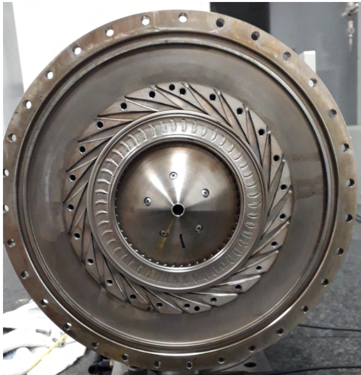
Figure 8: Photograph of the opened HT turbine with a view on the stator, rotor and exit cone.
