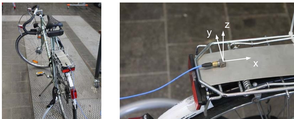
Figure 7: Experimental setup for measurement of ambient vibrations.
