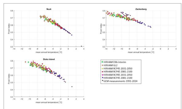
**Figure 2.** Frost index calculations from all model runs and from measurements against mean annual temperature for each station/corresponding grid cell. Green diamond: ERA Interim, orange diamond: historical, yellow dot: RCP 4.5 2031–2050, red dot: RCP 4.5 2081–2100, pink triangle: RCP 8.5 2031–2050, blue triangle: RCP 8.5 2081–2100, black star: GEM measurement 1991–2014.
