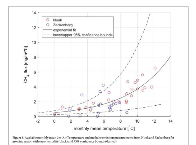
An exponential fit seems as a pragmatic option. The relationship between  $CH_4$  emission and temperature can now be used as a simple tool to upscale the potential methane fluxes for all of Greenland with the modelled temperature. This is based on the crude assumption that all of Greenland behaves like the two measurement stations available to us. The best-fitting exponential relationship is:  $C = 0.5206^* \exp(0.1960^*T)$  with T monthly mean temperature and C  $CH_4$  emission flux.
