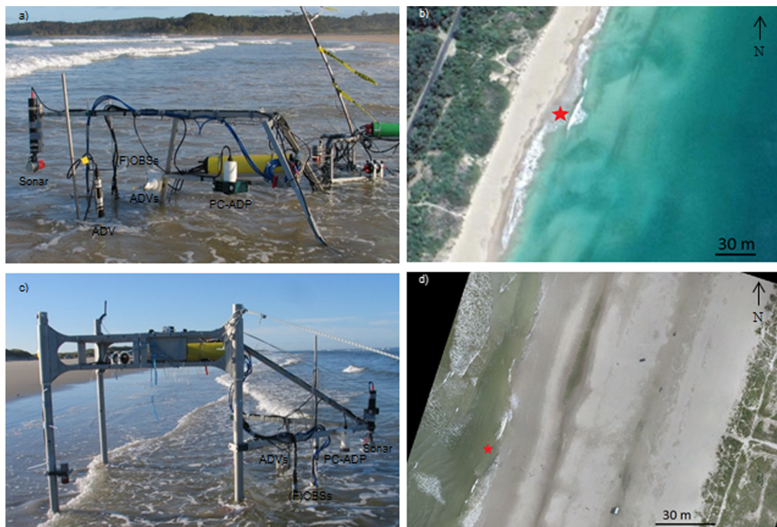
Figure 4. Photos of the instrument rigs during low tide at (a) Durras beach and (c) Vejers beach, and aerial photos of (b) Durras beach (Google Earth) and (d) Vejers beach (drone) during low tide. The positions of the instrument rigs are marked by red stars.
