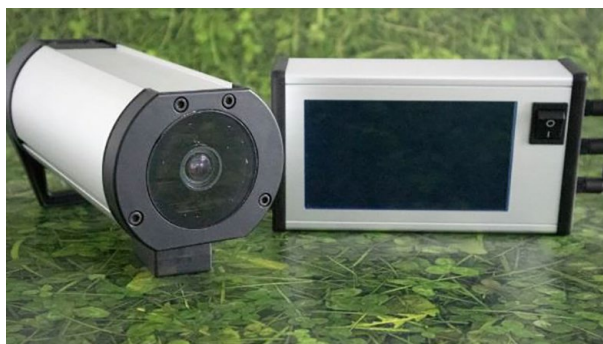
Figure 3. The Clovercam System by Agpointelli. A high-resolution RGB-camera and a processing terminal, displaying the current legume proportion.
