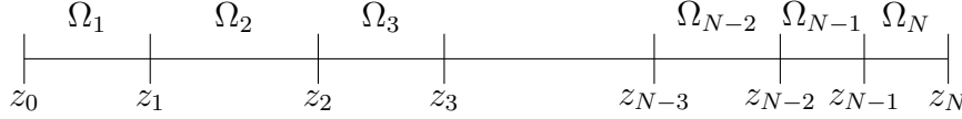
Figure 2.2.: Selected decomposition points z_0, z_1, \dots, z_{N-1}, z_N of the domain (z_0, z_N) . \Omega_1, \Omega_2, \dots, \Omega_N are the subdomains associated with the decomposition points.
