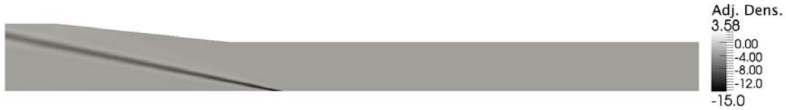
Fig. 7 Density contours for nominal conditions (inflow Mach number 5.0 and ramp angle 6.0^\circ )
