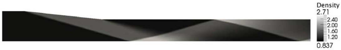
Fig. 7 Density contours for nominal conditions (inflow Mach number 5.0 and ramp angle 6.0^\circ )
