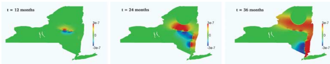
Figure 6. Effect of diffusion reduction normal to the river on the propagation front at (left to right) 12, 24, and 36 months: I_{\text{base}} - I_7 .
