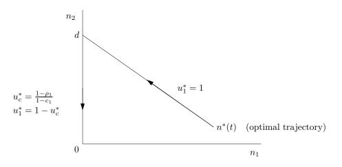
Figure 6: Optimal trajectory of the fluid control model when  $\rho_1 \ge c_1$ .
