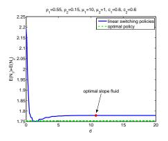
Figure 11: Mean total number of users for policies with a linear switching curve. The marker indicates the optimal slope for the fluid approximation.
