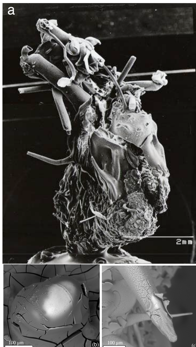
Figure 13: Chemical gardens grown in 0 g; SEM micrographs showing (a) growth under microgravity of a seed of a cobalt salt with sodium silicate. Reprinted with permission from ref 30. Copyright 1998 Elsevier. (b) \text{MnCl} in 6 M silicate. The brighter region is rich in \text{MnO}_2 and the darker in \text{MnSiO}_3 . (c) \text{NiSO}_4 in 2 M silicate, the external dark layer is \text{SiO}_n and the bright internal layer is nickel silicate. Reprinted with permission from ref 33. Copyright 2011 American Chemical Society.
