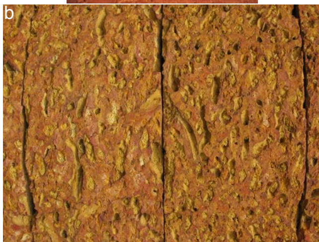
Figure 38: (a), Laterite quarry in Angadipuram, India. Image from Werner Schellmann. (b), close-up view, which spans about 1 dm vertically, of typical laterite showing tubular structures surrounded by various iron oxides. Image from Phó Nháy.
