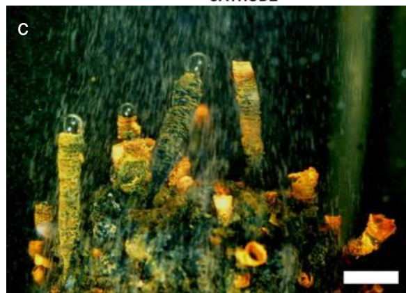
Figure 21: (a) Curved tubes approximately 1 cm long of precipitating magnetite, with an outer layer oxidized to orange lepidocrocite, grown on a negatively charged magnet in a solution of iron(III) ammonium sulfate. (b) Schematic diagram of the bubble and tube walls growing on the cathode. (c) Growing tubes with bubbles emerging (scale bar = 5 mm). Reprinted with permission from ref 44. Copyright 2004 National Academy of Sciences, USA.
