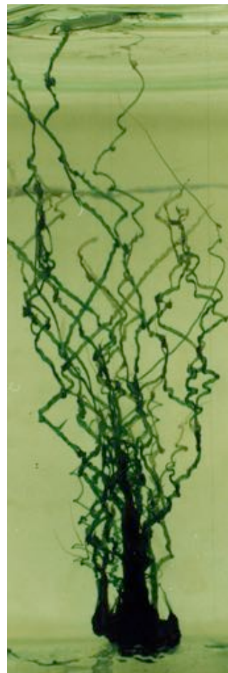
Figure 14: A cobalt sulfate chemical garden grown at 1 g with sodium silicate displays tubular growth deviating from the vertical by preferred angles; a phenomenon as yet unexplained. The size is some tens of centimeters. Image from David Jones.
