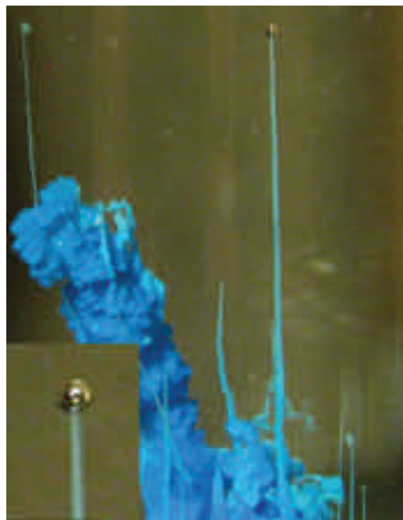
Figure 9: Tube growth with a bubble at the tip; the inset photo shows a magnified view of an air bubble during the vertical growth process. Field of view: 1.9 \times 2.5 cm; inset: 2.4 \times 3.2 mm. Reprinted with permission from ref 52. Copyright 2005 The Royal Society of Chemistry.
