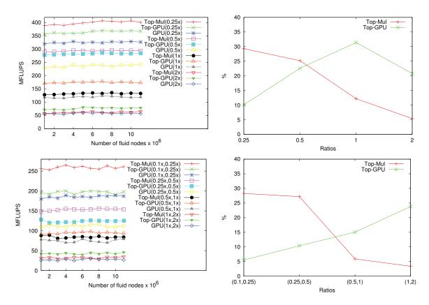
Figure 4. One refined level (top) and Two refined levels (bottom). Performance (left), in terms of MFLUPS, achieved by the three approaches, homogeneous GPU, heterogeneous *Top-Multocore* and heterogeneous *Top-GPU*. Gain (right), in terms of percentage, of each of the both heterogeneous implementations, *Top-Multicore* and *Top-GPU*, against the homogeneous GPU implementation.
