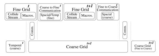
Figure 2. Steps of the multi-domain LBM code for our heterogeneous (Multicore-GPU) approach.
