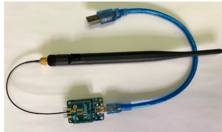
Figure 10. Receiver: Xbee card with antenna and USB cable.
