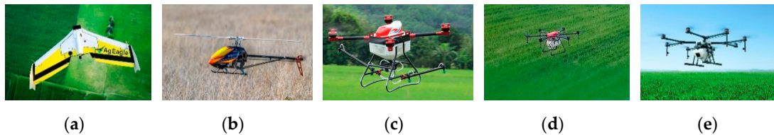
Figure 1. RPAS (remotely piloted aircraft system) types: Fixed-wing (a). Single-rotor (b). Quad Copter (c). Hexa Copter (d). Octo Copter (e).
