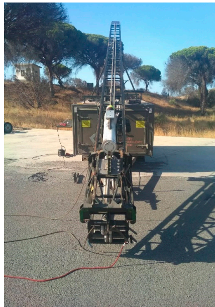
Figure 14. Detail of the QuinetiQ© Energy Catapult launcher with a dummy on the ramp.
