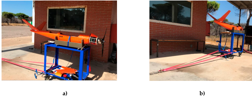
Figure 13. Modified electric ALO in thrust test bench. (a) lateral view, (b) stern view
