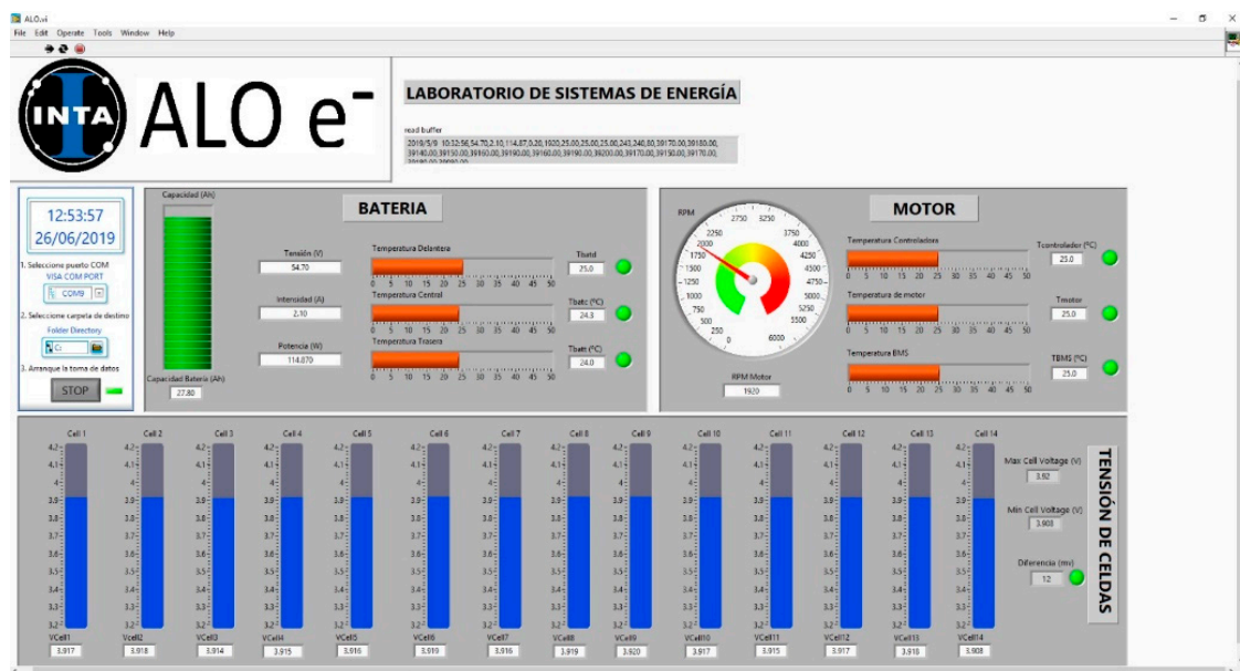
Figure 11. Developed SCADA software for electric ALO platform.
