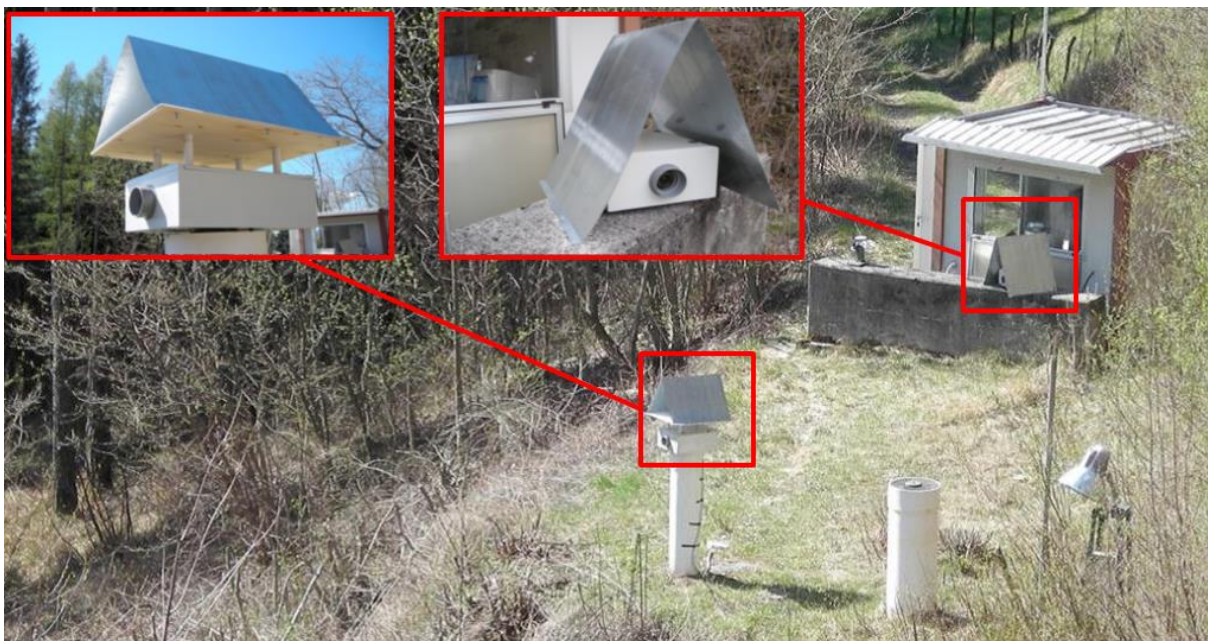
Fig. 4. The monitoring station at Moda when it was equipped with a stereo-photogrammetric setup (Antonello et al, 2013).
