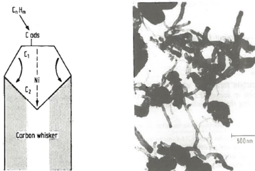
FIGURE 1.8: Whiskers growth by diffusion through nickel particles (left) and electron micrograph of whisker-like carbon formed by decomposition of methane on nickel catalyst at 500 °C (right) [12].
