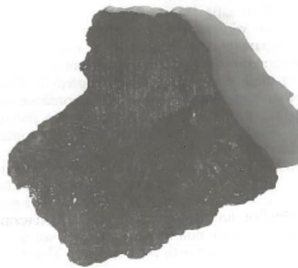
FIGURE 1.10: Coke deposit formed by pyrolysis of light paraffins. The coke was deposited in tubular reformer operating with nearly inactive catalyst at the inlet [12].
