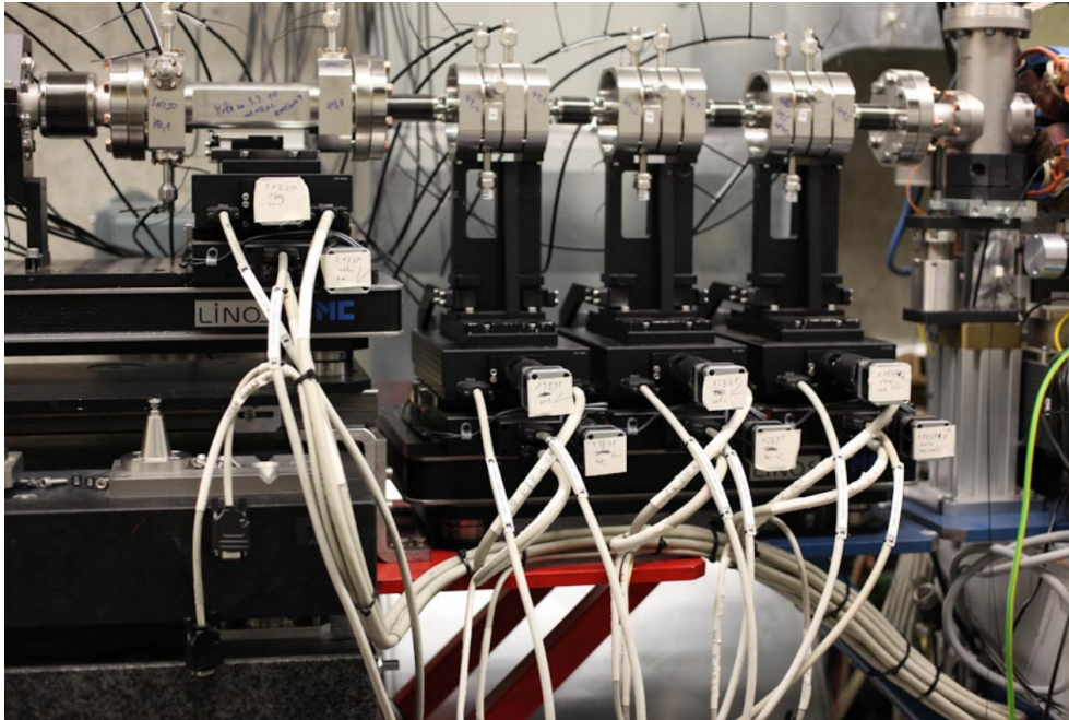
Figure 6.1: Cavity BPM test-stand at FLASH1 with three EU-XFEL “undulator” Cavity BPMs (on the right) on remote movers. An EU-XFEL “beamline” Cavity BPM is also installed, but it was not used during the tests (on the left).
