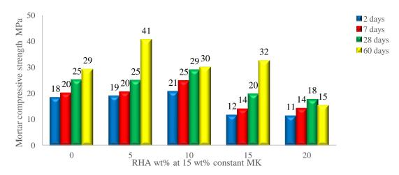
Figure 17 – Effect of RHA content at constant 15 wt% MK on compressive strength of blends and OPC mortars
