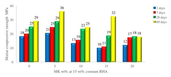
Figure 13 - Effect of MK content on mortar strength of blends at constant 15 wt% RHA and OPC
