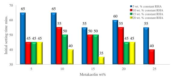
Figure 7 – Effect of MK content at constant RHA content on initial setting time of ternary blends
