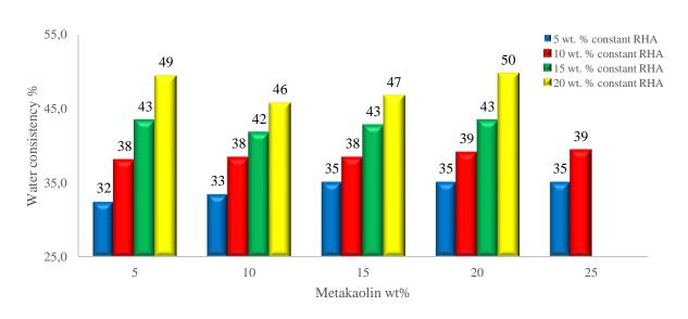
Figure 3 - Effect of MK at constant RHA on the consistency of ternary blend
