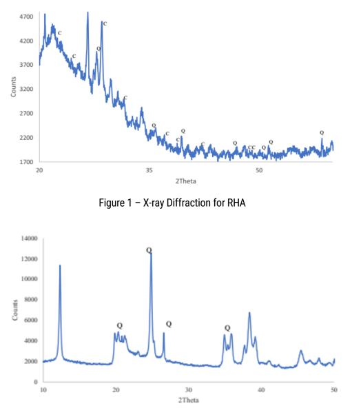
Figure 2 - X-ray diffraction for MK
