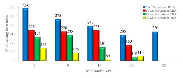
Figure 8 - Effect of MK content at constant RHA content on final setting time of ternary blends
