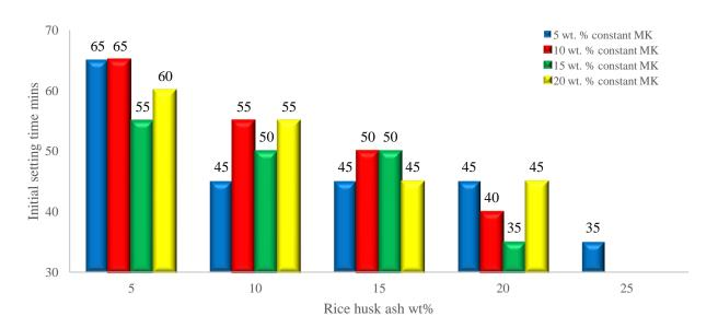
Figure 5 - Effect of RHA content at constant MK content on initial setting time of ternary blends
