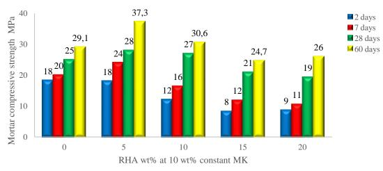
Figure 16 - Effect of RHA content at constant 10 wt% MK on compressive strength of blends and OPC mortars
