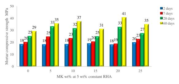
Figure 11 - Effect of MK content on Strength of blends and OPC mortars at 5 wt% constant RHA
