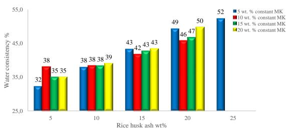
Figure 4 – Effect of RHA at constant MK on consistency of ternary blend
