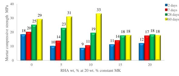
Figure 18 - Effect of RHA content at constant 20 wt% MK content on Strength of blends and OPC mortars
