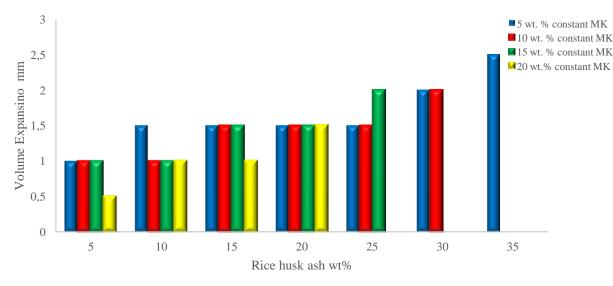
Figure 9 - Effect of RHA content at constant MK content on volume expansion of ternary blends
