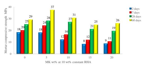
Figure 12 - Effect of MK content on mortar strength of blends at constant 10 wt% RHA and OPC
