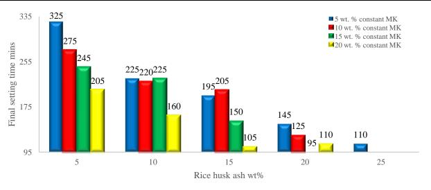
Figure 6 - Effect of RHA content at constant MK content on final setting time of ternary blends
