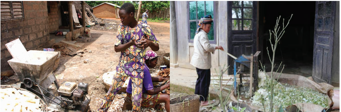
Small-scale simple machinery and equipment can significantly help women save their time and labor. Left: a cassava milling machine in Benin. Photo: D. Dufour. Right: a sweet potato vine cutting machine for animal feeding in Vietnam. Photo: Nguyen Thi Van Anh.
