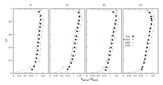
Figure 2: Mean streamwise velocity of the continuous phase for different turbulence models in Mesh A.
