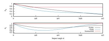
Figure 12: Values of the normal  $(e_n)$  and tangential  $(e_t)$  restitution coefficients.
