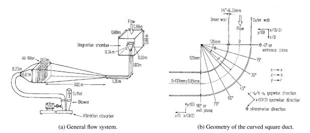
Figure 1: Experimental set-up of the experiment carried out by Kliafas and Holt. 16
