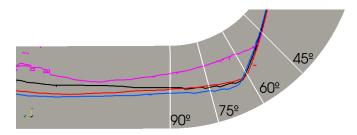
Figure 11: Isolines with mean volumetric fraction  $\alpha_{vf} = 1 \times 10^{-9}$  at mid-plane for cases: elastic (black),  $R = 1 \times 10^{-6}$  (red),  $R = 1 \times 10^{-9}$  (blue) and  $R = 1 \times 10^{-5}$  (pink).
