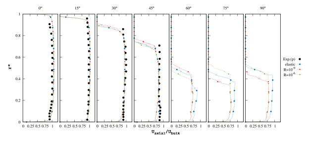
Figure 9: Results comparing elastic vs. inelastic collision modelling for particle-wall collisions.
