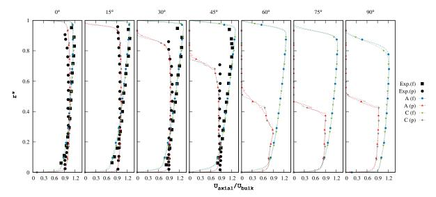
Figure 5: Results for continuous and dispersed phases comparing meshes A and C (inlet BC: turbulent).
