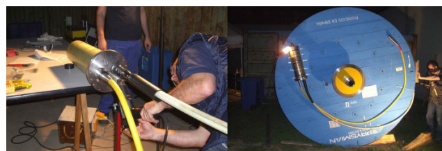
FIGURE 4. Left: Termination box. Right: Cable deployment with termination box unit.
