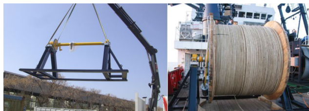
FIGURE 6. Reel with the 4km cable and its support for deployment.
