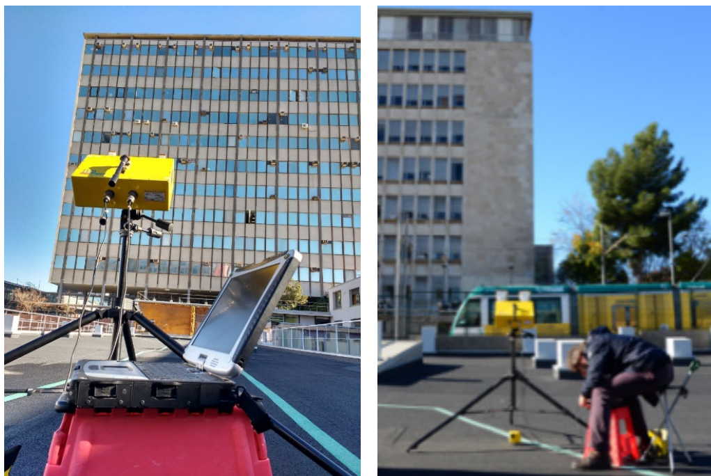
Figure 1: Remote sensing with RAR, building A (left) and building B (right).
