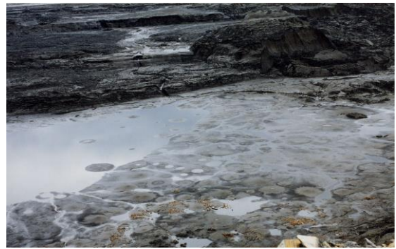
Figure 27. Evidence of tailings liquefaction
