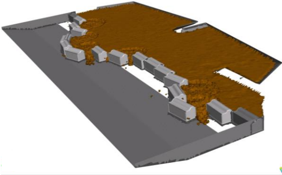
Figure 45. Computed caisson locations at the end of failure from the PFEM analysis
