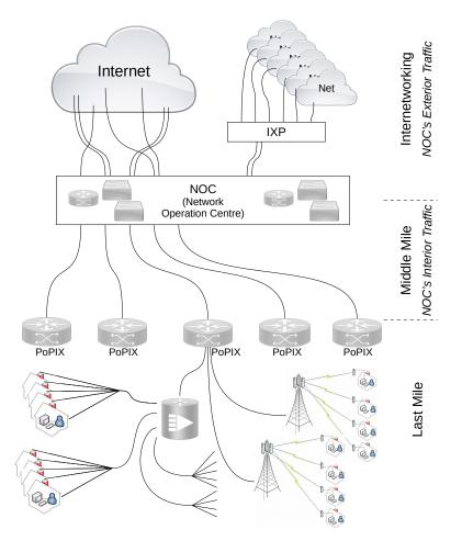
Figure 1: The Guifi.net network architecture.
