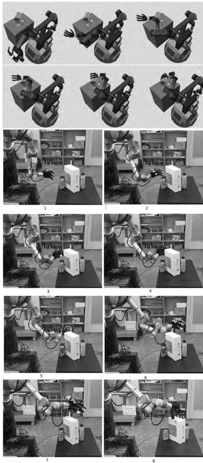
Fig. 12. Snapshots of the grasping of a box in simulation and in the real environment.
