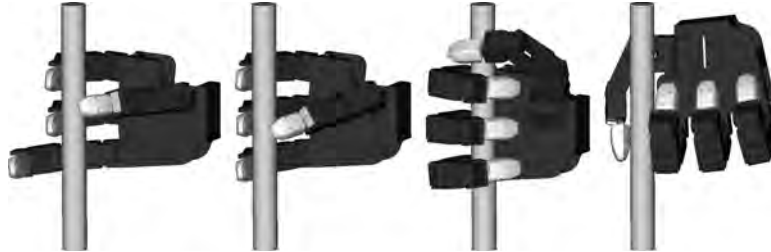
Fig. 9. Examples of grasps of each family used to grasp a cylinder: Thumb-2 Finger , Thumb-3 Finger , Medium Wrap and Lateral Pinch (from left to right, respectively).
