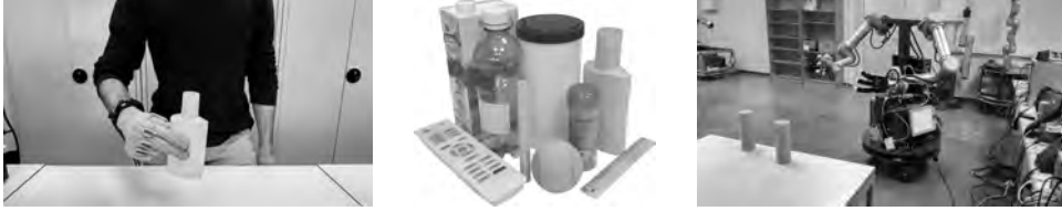
Fig. 1. Human operator wearing the measurement equipment (left), set of grasped objects in the experiments (middle), and dual-arm robot (right).
