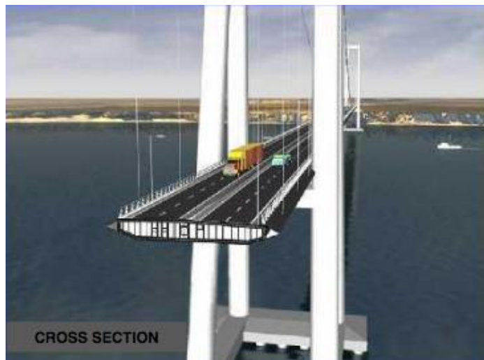
Figure 4.15 Bridge cross section.
