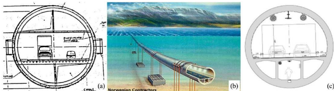
Figure 2.5 SFT with circular cross section. (a) Messina Strait crossing (Italy) proposed by ATI-SSST (Scolari et al., 1989); (b) Høgsfjord crossing (Norway) proposed by Aker Norwegian contractors (Skorpa and Østlid, 2001); (c) Sulafjord crossing (Norway) (Jakobsen et al., 2009).
