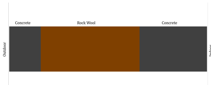
Figure 3.1: Load bearing wall structure (lateral cross-section view)
