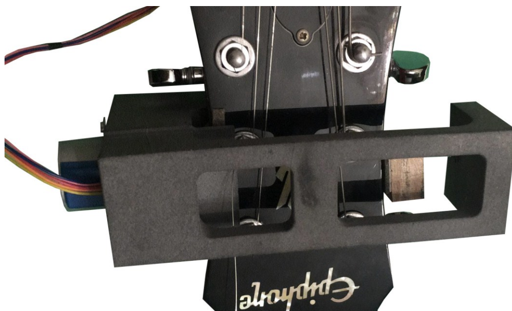
Picture 35. Tuning structure installed on a guitar
