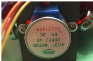
Picture 36. Detail of motor assembly to the structure
