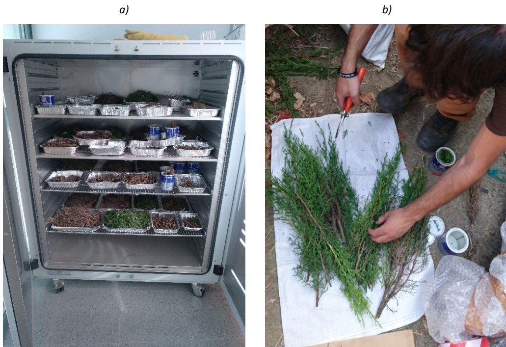
Figure 4. a) Fuel separated in different classes before oven-drying; b) Fuel moisture content sampling
