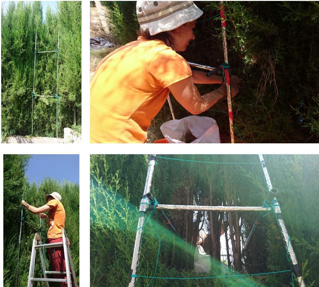
Figure 2. Tubing structure used to define the volumes of interest. 0.5 \times 0.5 \text{ m}^2 surface delimited by the vertical tubes and the green threads.
