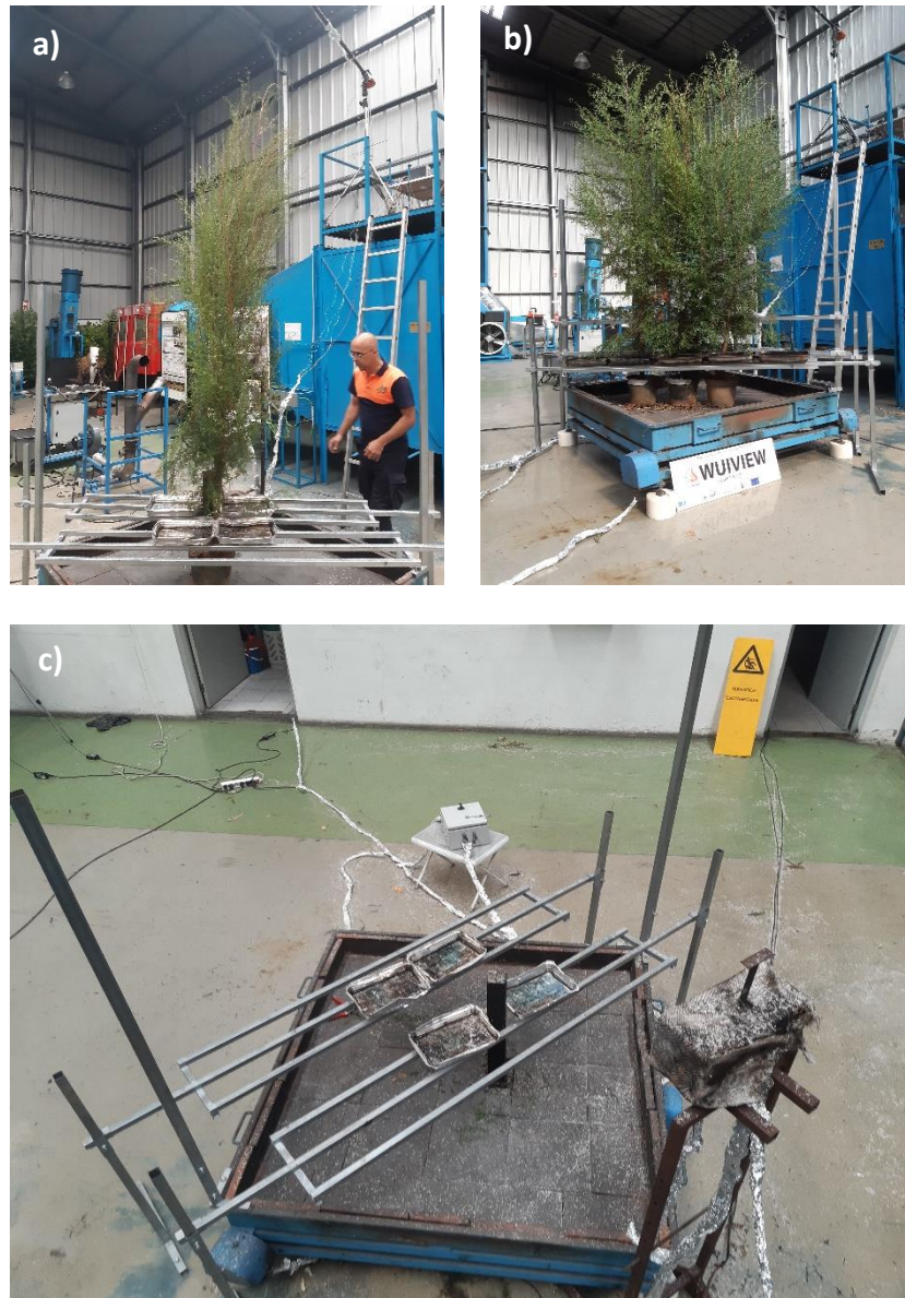
Figure 3. (a) Single-tree configuration (4 ignition trays distributed under the canopy base); (b) Three-trees configuration (9 ignition trays distributed under the canopy base); (c) Load cell module and structures to hold ignition trays.
