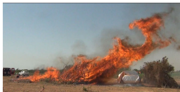
Figure 5. Video snapshot acquired 4min 03sec after ignition, showing highest car exposure to flames.
