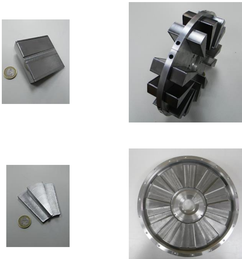
Figure 4. Stator pole piece (upper left) and stator with stator poles inserted into the aluminum structural disk (upper right). Rotor pole piece (lower left) and view of the rotor pieces glued in the cover (lower right).
