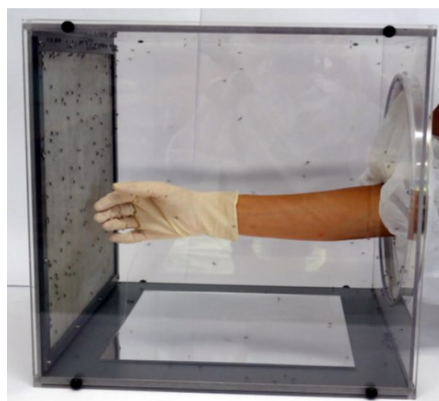
Figure 6: The arm-in-cage (AIC) test for measuring the efficacy of topical mosquito repellents under laboratory conditions [45].
