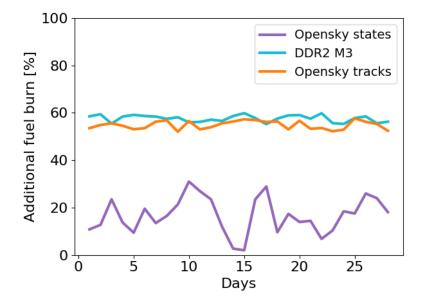
Figure 4: Additional fuel burn (in percent per day) due to inefficient vertical profiles, calculated as the difference between the actual flown trajectories (DDR m3, Opensky tracks or Opensky states) and the optimal trajectories, in total fuel consumption per day inside TMA for the month of February 2018.
