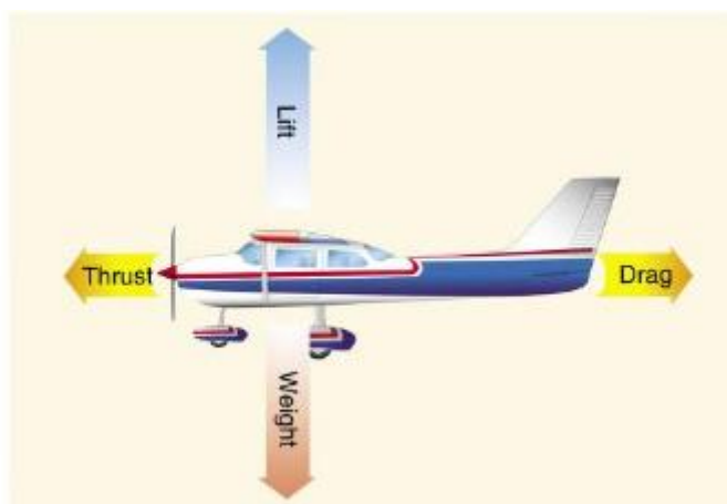
Figure 7.2: Relationship of forces acting on an airplane. Source: [Federal Aviation Administration, 2009]
