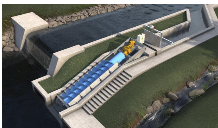
Figure 3.3 Archimedes screw as a generator [8]
