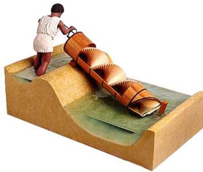
Figure 3.1 Screw used as a pump for irrigation [5]
