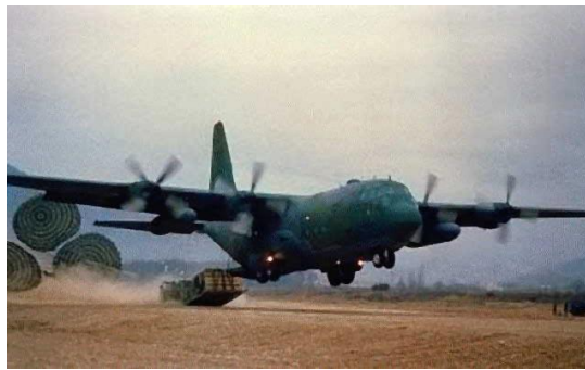
Figure 4: C-130 Hercules dropping pallet with Low Altitude Parachute Extraction System on Khe Sanh runway. Retrieved from [9]
