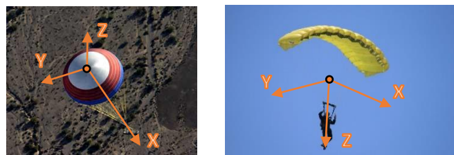
Figure 17: On the left, body axes represented for a conventional parachute. On the right, body axes represented for a ram-air parachute. Retrieved from [44, 45]
