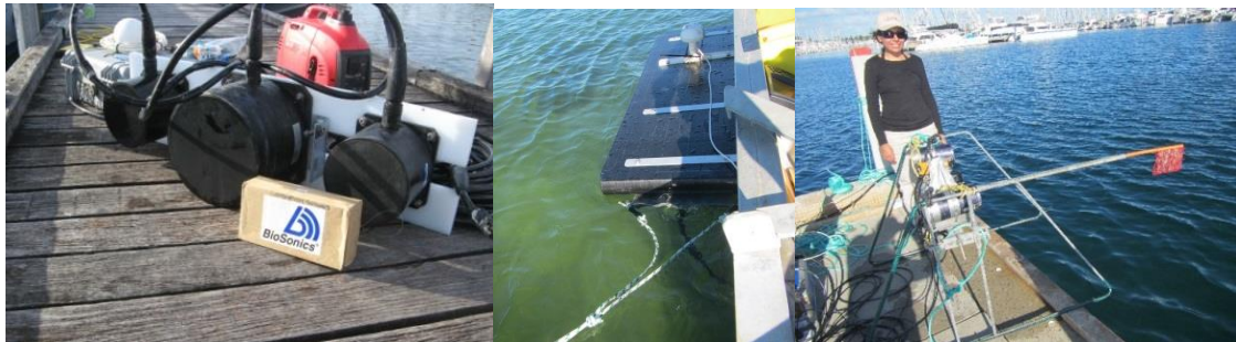
Figure 5.3. Three echo-sounders were mounted in a pontoon which was towed on the side of the vessel (left and centre). One of the Stereo-BRUVS used in the experiments is shown on the right of the figure.
