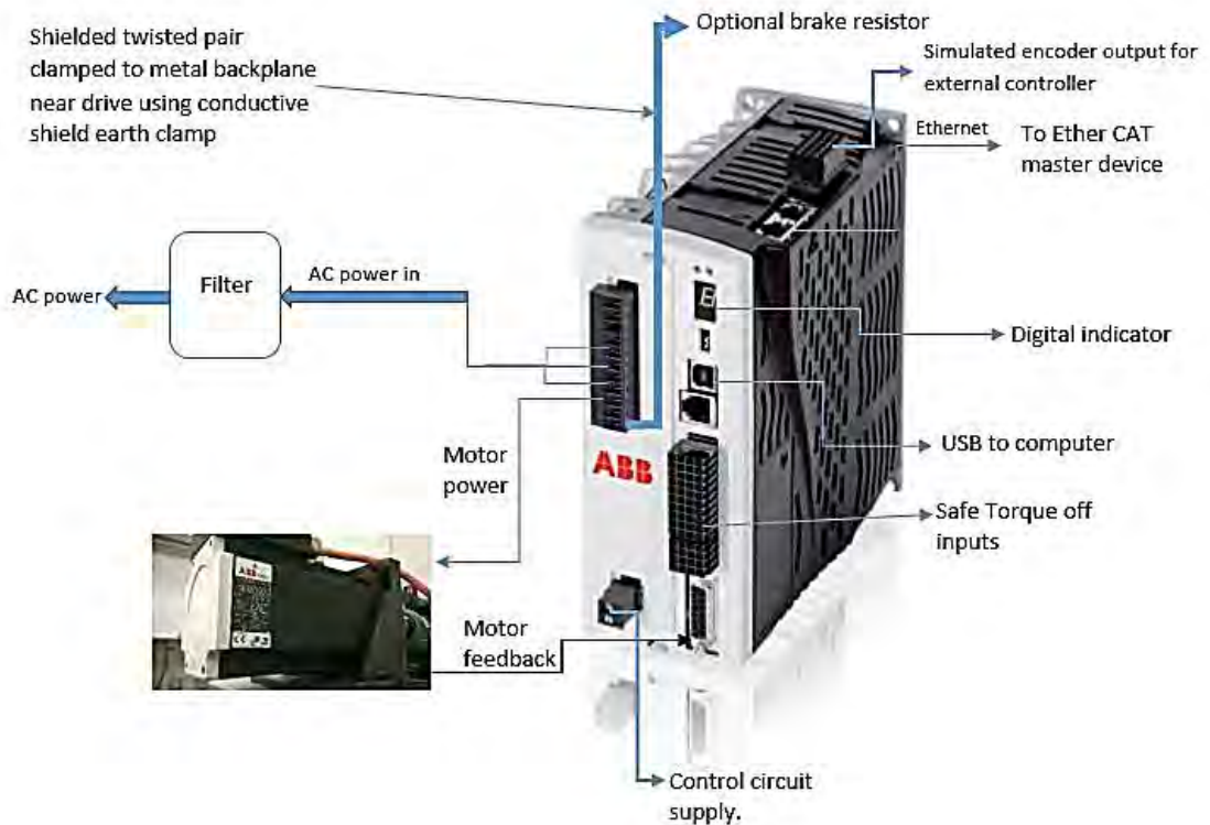
Figure 3.4 Diagram of MicroFlex e150 servo drives with the connections(ABB, 2012).
