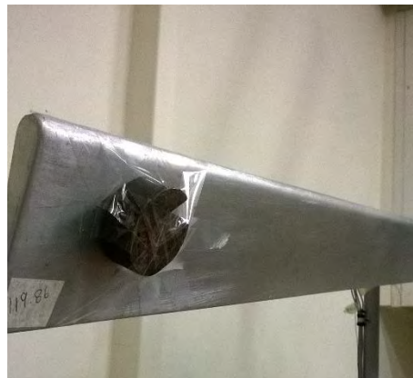
Figure 3.22 The blade model during imbalance test (adding 200g mass).
