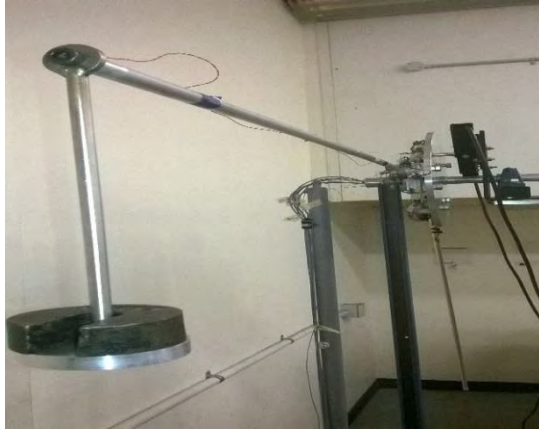
Figure 3.15 Strain gauge calibration test with weight holder
