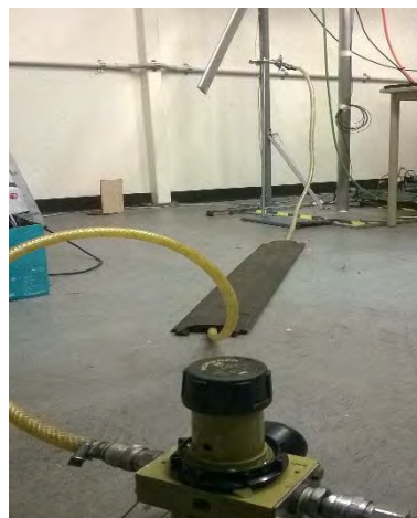
Figure 3.23 Compressed air system for providing a variable air burst towards upwind and downwind.
