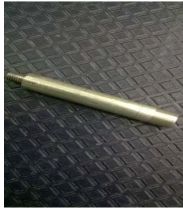
Figure 3.17 The Aluminium optional extension part of 35mm long and 14.95g
