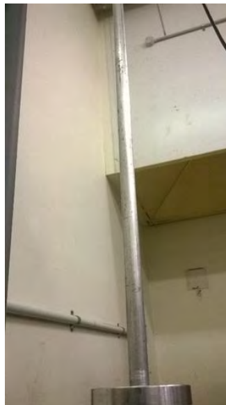
Figure 3.16 The rotating beam in the vertical position with experiment mass screwed in the end.
