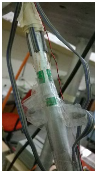
Figure 3.6 Rotating beam instrumented with three groups of strain gauges
