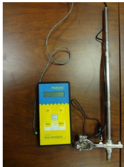
Figura 3.18 Micro molinete – Aqua Count
