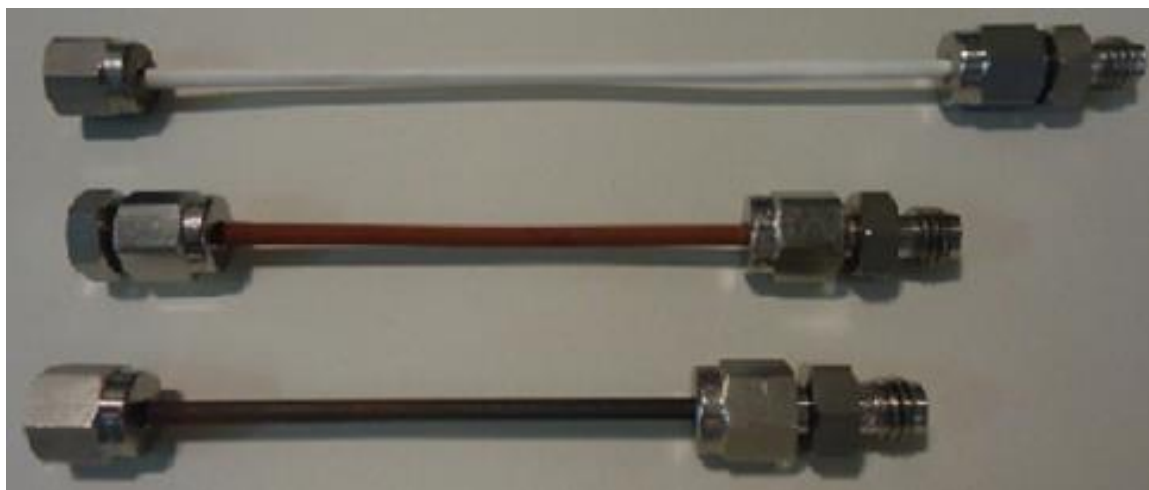
Figura 1. Picture of different CMRs: Top, hollow fiber used for the blank tests; Middle, CMR with iron and cerium oxide; Below, CMR with three phases, iron and cerium oxide and palladium.
