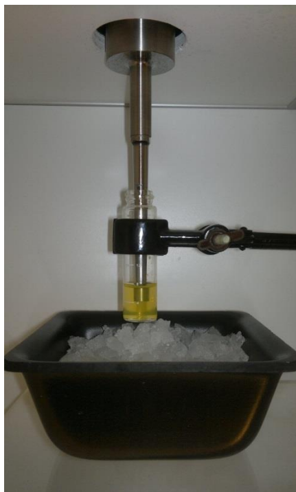
Figure 2: Photograph showing recommended positioning of probe sonicator in sample
