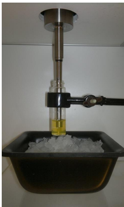
Figure 3: Photograph showing recommended positioning of probe sonicator in sample
