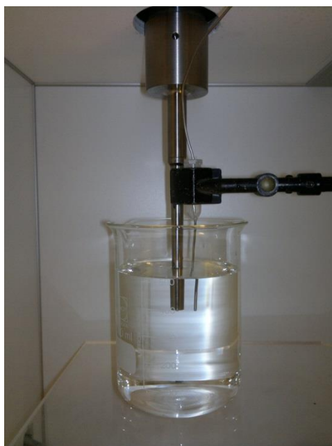
Figure 1: Photograph of probe sonicator and thermocouple positioning for calorimetric calibration (thermal insulation removed for clarity)
