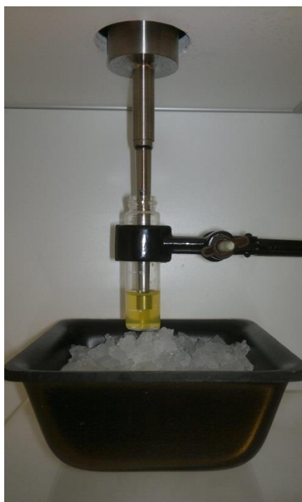
Figure 2: Photograph illustrating the mounting of probe sonicator in sample
