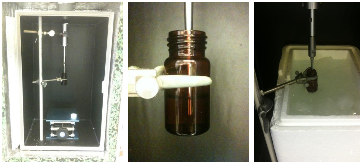
Figure 2: Ultrasonic probe sonication setup for dispersion of NM powders
