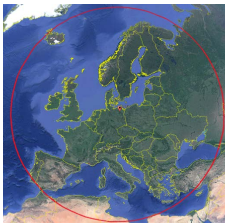
Figure 8: Receiving mask of the DLR ground station in Neustrelitz, Germany.
