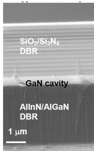
Fig. 5.3 - 3\lambda/2 bulk GaN cavity surrounded by a bottom AlInN/AlGaN Bragg mirror and a top dielectric mirror
